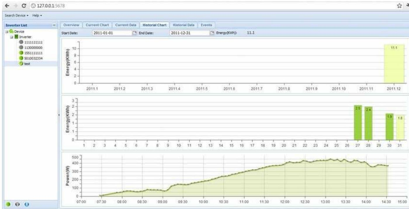
**Notes:** If select the “Inverter” option in Inverter List panel it will display the total energy generation data or power curve of all inverters.
