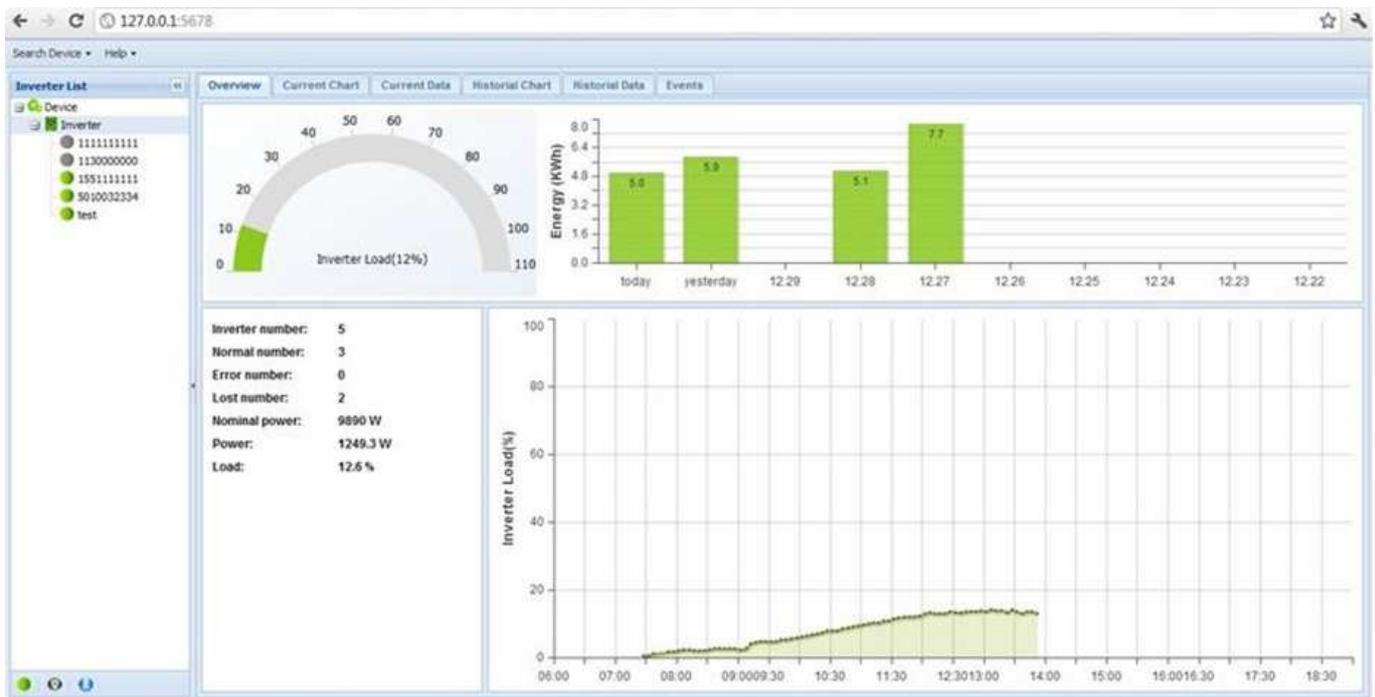
1. The dashboard on the upper left corner shows the load percentage of inverter (actual output power/nominal output power). When users select the “Inverters” option in the Inverter List panel the dashboard will represent the total load percentage of all the inverters, while choose one of the inverter in the Inverter List it will be the load percentage of the selected inverter.
